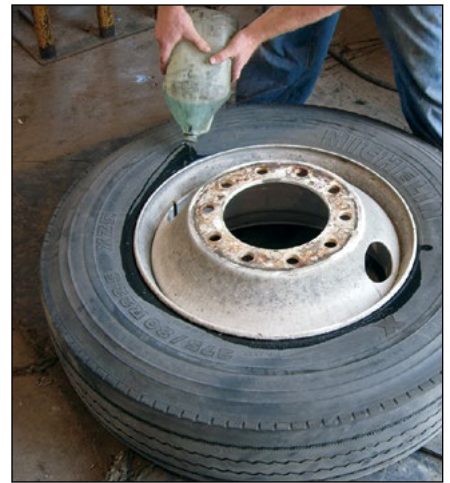
3 Lubricate both beads completely to avoid demount damage.
