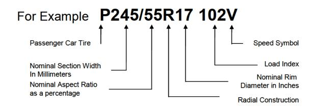
**Load Index Number,** a numeric code which indicates the maximum load carrying capacity of a tire at the maximum cold inflation pressure.
