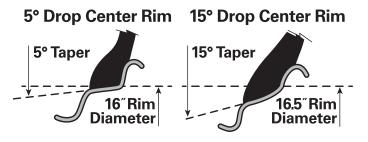
The following diagram shows how the beads of a 16" tire will not seat on a 16.5" rim. The beads should not be forced out against the rim flanges by using more air pressure, because this will break the beads and the tire will explode. Never exceed 40 psi when seating the beads on the rims.
