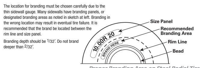
Proper Branding Area on Steel Radial Tire
