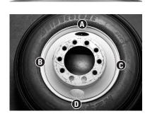
7. Distances A, B, C, and D should be within 2/32". If they are not, break down, re-lubricate and mount again.
