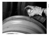
2. Protect bare metal with primer or anti-rust paint to prevent further corrosion. Allow to dry.
