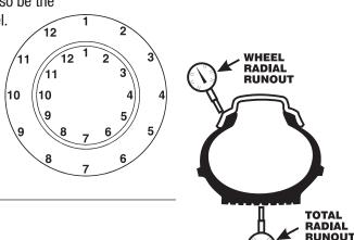
Proper Position for Measuring Runout
