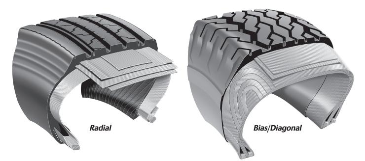
Radial tire body ply cords are placed straight across the tire from bead to bead. In addition, radial tires have belt plies, which run circumferentially around the tires, under the tread. They constrict the radial ply cords and stabilize the tread area.
