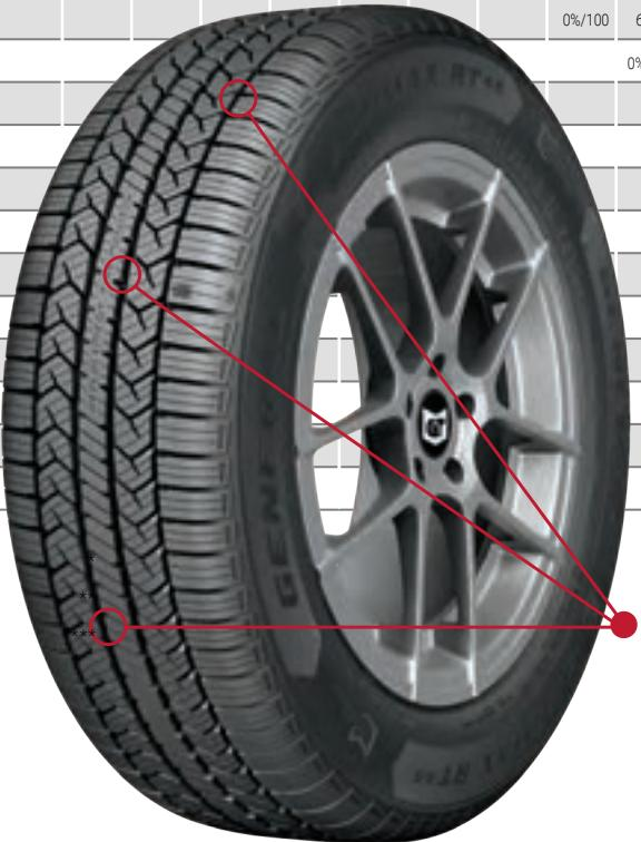
Dot shows an example of where to take measurements. It is NOT recommended to measure straight across in one location.
