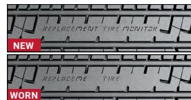
Letters in the tread wear off to read "REPLACE TIRE" when the tire wears to 2/32 of tread depth, indicating a tire change is needed.
