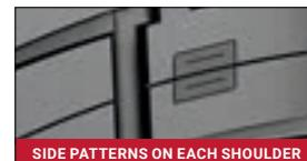
Indicators in both sides of the tread wear off evenly, ensuring the driver of proper alignment, or wear off unevenly, alerting the driver to check the wheel alignment.
